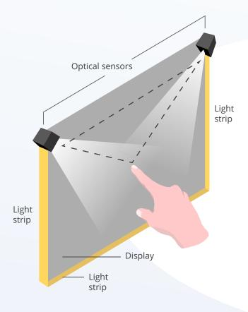
In addition, optical touch displays tend to last for a long time because the light touches associated with this tech variant do not generally result in wear and tear.
