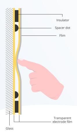
The cost of resistive touch is generally on the lower side when compared to different touch panel technologies, making them a good option for simple, single point touch applications.
