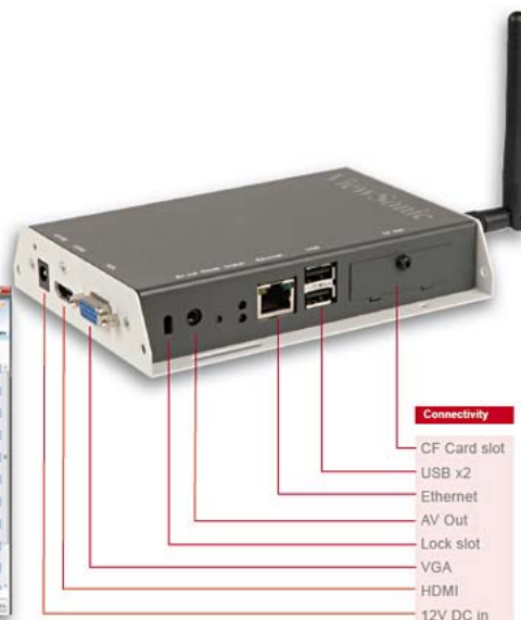
Rugged metal housing VESA compatible mounting bracket
