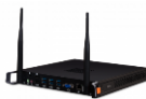
VPC16-WP-3 Slot-In-PC CPU Core®i5 8500 (vPro, TPM, UNITE®); 8GB RAM; 128GB SSD EAN 76690700320 8
