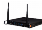
VPC17-WP Slot-In-PC CPU Core®i7 8700 (vPro, TPM, UNITE®); 8GB RAM; 128GB SSD EAN 76690700322 2
